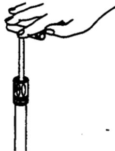
2. If a cartridge case is in the chamber, tap it out with a cleaning rod.
