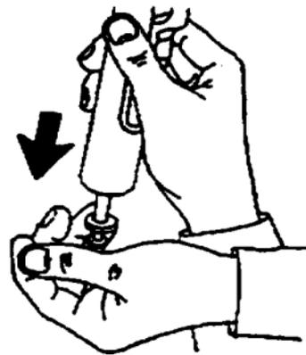
15. Drop firing pin out rear of bolt carrier.
