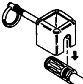
2. Hook behind first groove of compensator.
