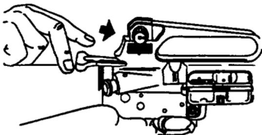
3. If cartridge or case is ejected or chamber is clear, Release charging handle to feed new round. Don't ride the charging handle forward.
