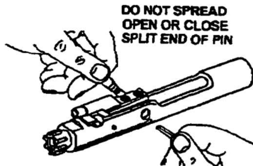
13. Remove firing pin retaining pin.
