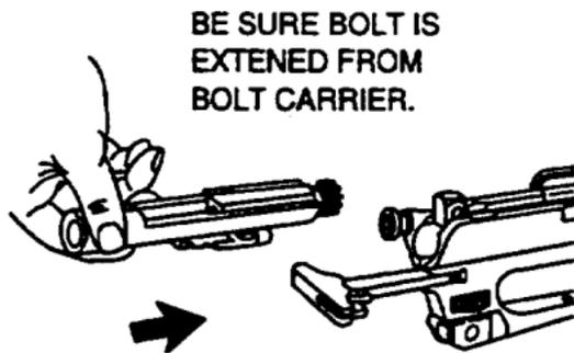
12. Slide in bolt carrier assembly.
