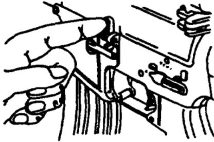
e. Depress upper portion of bolt catch. Bolt should go forward.
