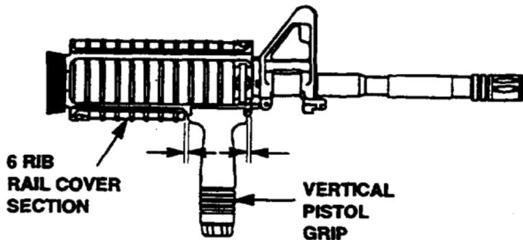
2. For the carbine, if the pistol grip will be installed at the muzzle end of the rail, first install a half length "6 rib" rail cover section so it latches into the end slot.
