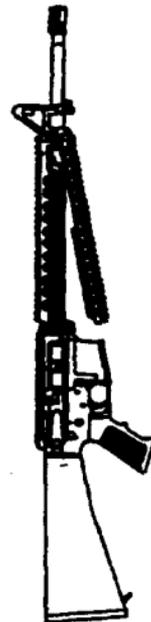
4. The recoil slots of each rail are sequentially numbered within the recoil slots themselves. The recoil slots of the top rail have a "T" prefix while those of the bottom rail have a "B" prefix. The recoil slots of the left rail have an "L" prefix, and the right rail have an "R" prefix. The numbers and prefixes are provided to assist in remounting an accessory in the same position if removed.
