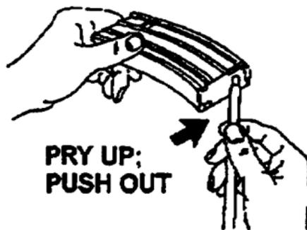
1. Release base catch with end of a cleaning rod.
