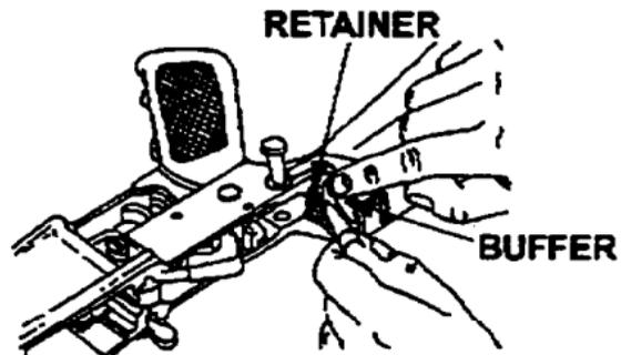
20. Press in buffer, depress retainer, and release buffer.
