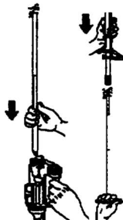
**START AT RECEIVER AND DROP ROD THROUGH.**
