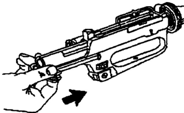
13. Push charging handle and bolt carrier assembly together into upper receiver until fully seated.
