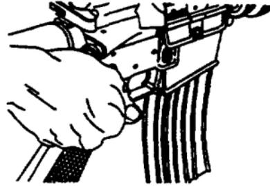
f. Tap forward assist to ensure bolt is fully forward and locked.
