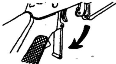
1. To operate the weapon in extreme cold, depress the trigger guard plunger and open the trigger guard to obtain easy access to the trigger when wearing Arctic mittens.
