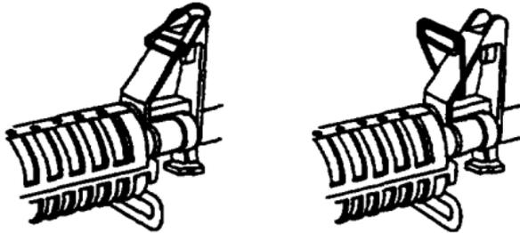
2. Work adapter sling through swivel and through loop.
