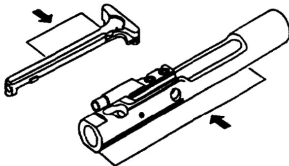
3. Lightly lube charging handle and inner and outer surfaces of bolt carrier. Generously lube slide and cam pin area of bolt carrier.
