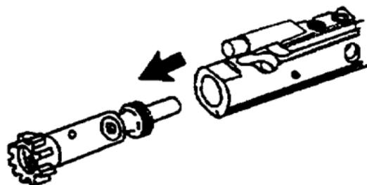
17. Remove bolt assembly from carrier.
