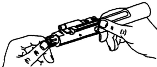
14. Push in bolt assembly to locked position.
