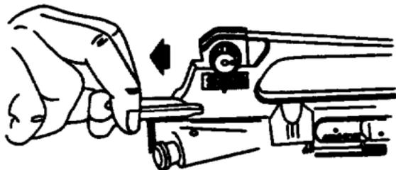
g. Chambering a round from the bolt closed position; with magazine inserted, pull charging handle fully rearward.
