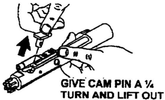
16. Remove bolt cam pin.
