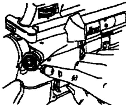
17. Close upper and lower receiver assembly. Push in takedown pin.
