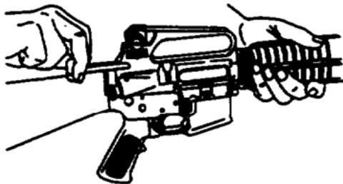
1. If your weapon still fails to fire after performing. Immediate Action. check again for jammed cartridge case.
