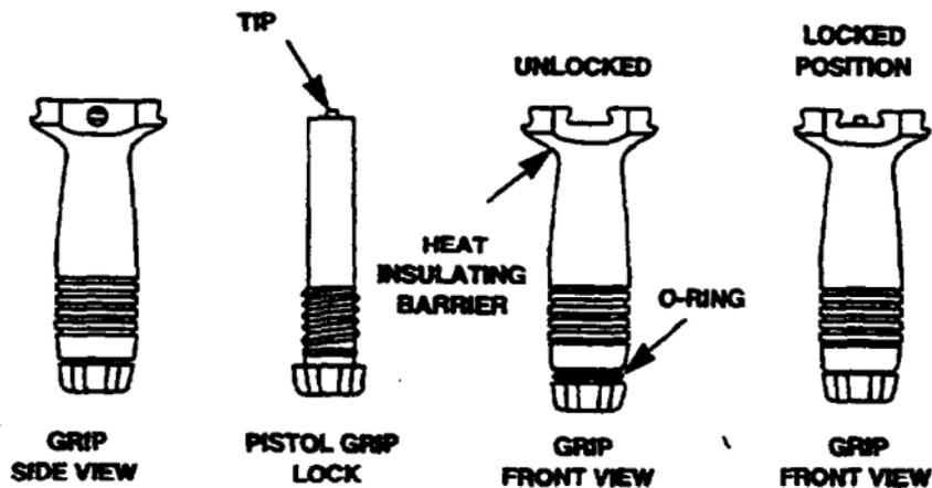
4. Unscrew the pistol grip lock to the point that the upper tip rests below the slotted surface of the base in the unlocked position.
