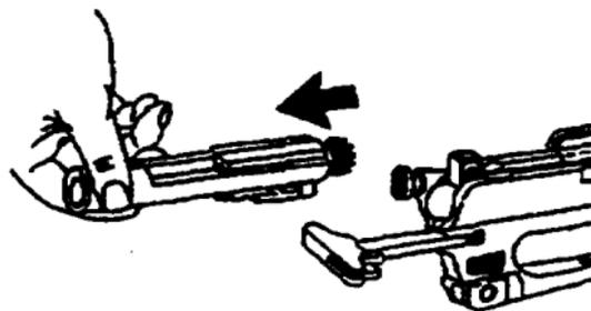
11. Remove bolt carrier and bolt.
