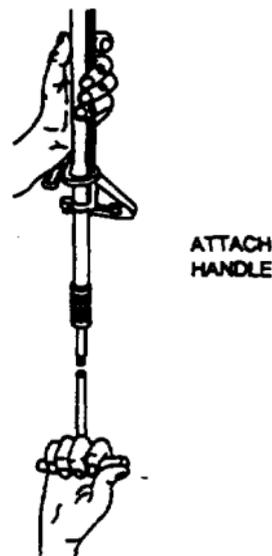
8. Send a patch through the bore once in a while to help clean out the crud that the brush is getting loose. Replace the bore brush with the rod tip (patch holder) and a wet patch. Drop it through. You won't need to attach the handle to pull only a patch through.
