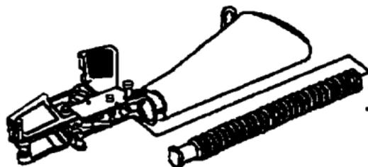
1. Grasp the lock release lever in the area of the retaining nut and pull to reinstall the buttstock assembly onto the lower receiver extension.
