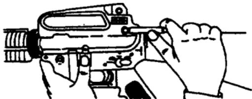
3. To lock bolt open, pull charging handle rearward. Press bottom of bolt catch and allow bolt to move forward until it engages bolt catch. Return charging handle to full forward position. If you haven't before, place selector lever on SAFE.
