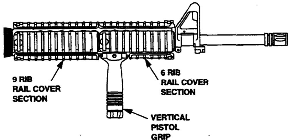
3. For the rifle, first install a "9 rib" rail cover, next the vertical pistol grip and then a "6 rib" rail cover. The pistol grip may be moved to the muzzle end, if desired.
