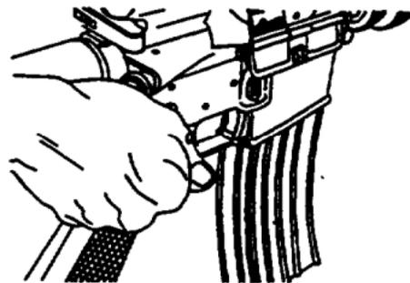
4. Release charging handle and strike forward assist to seat round end lock bolt.
